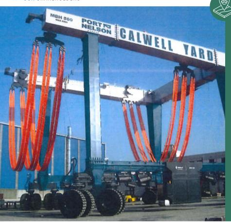
// Standing at 18 metres tall, the travel lift will lift vessels up to 550 tonnes. This hoist will give the operation greater flexibility and will provide the benefit of being able to lift and store multiple vessels onto our hardstand area.
